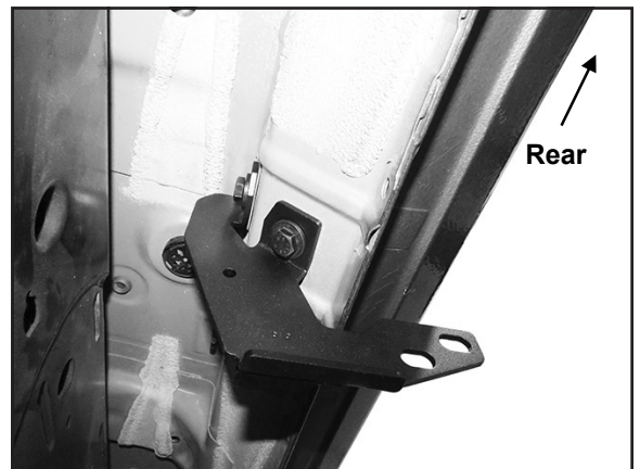
(Figure 9) Passenger/right Rear Bracket installed.
